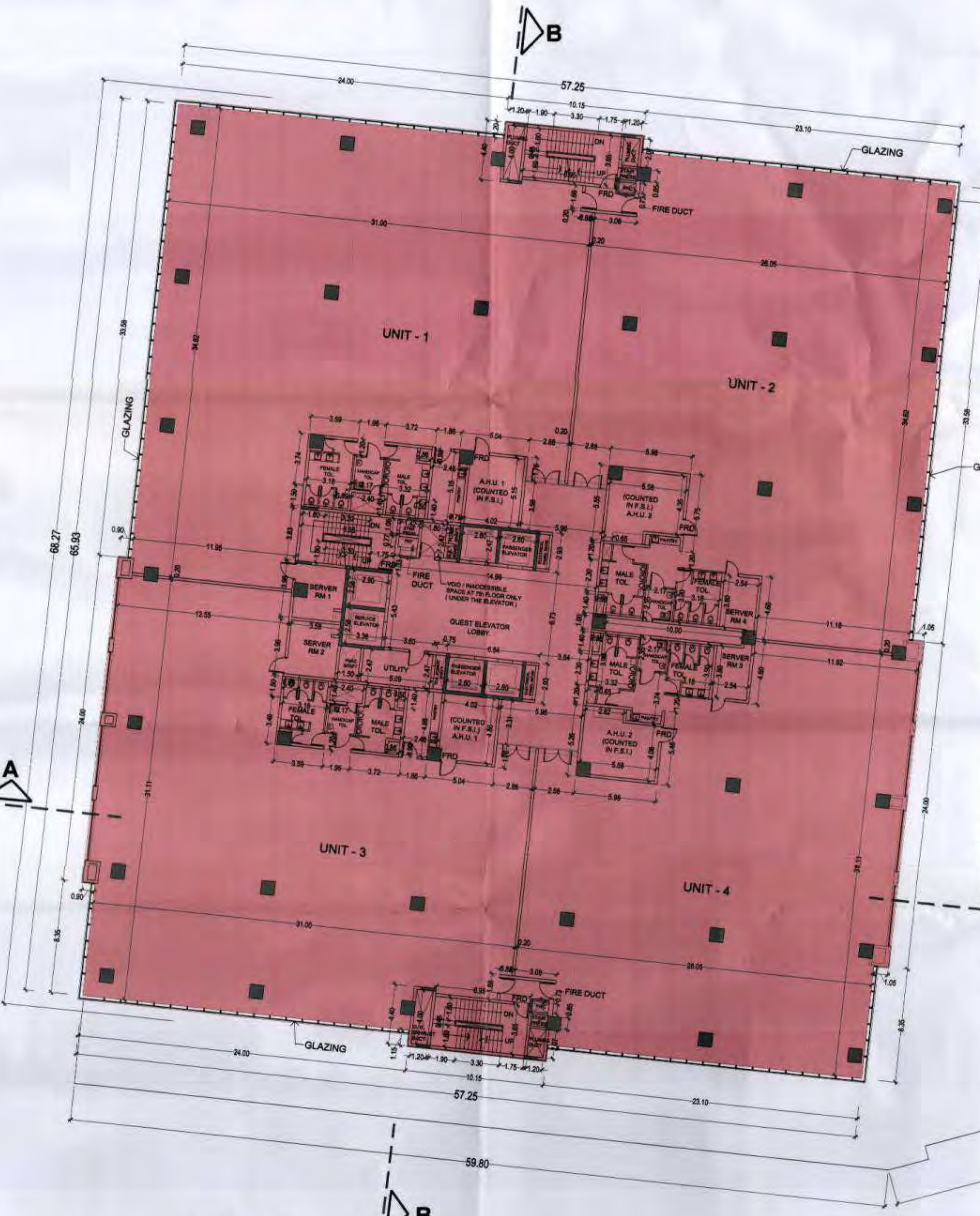
3RD, 4TH, 5TH & 7TH FLOOR AREA DIAGRAM OF WING 'A' SCALE: 1:250
